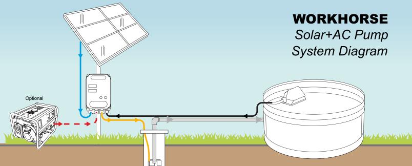
W10-350 Deep Pump W25-100 High Volume Pump For use with 800w - 2000w Solar Array or AC Backup Up to 400ft of head with DEEP series and up to 70GPM with VOLUME series.
