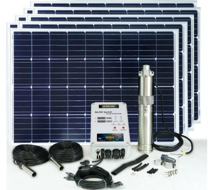
The **800** delivers power and versatility. It comes standard with **eight 100 watt solar panels**, a 'smart' controller, wires and sensors. It operates at a **maximum head of 328 ft** and generates flow rates up to **9.2 gallons per minute**. The **800V+** with centrifugal pump is a higher volume, lower head option delivering up to **16GPM** at low heads.
